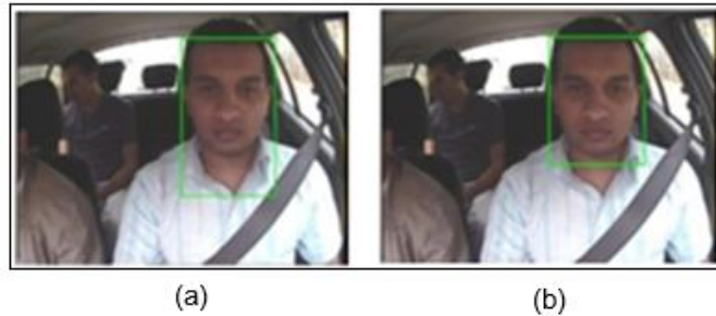
Fig 6. Elimination of the neck area from the face. (a) Result before the operation, (b) Result after the operation.
