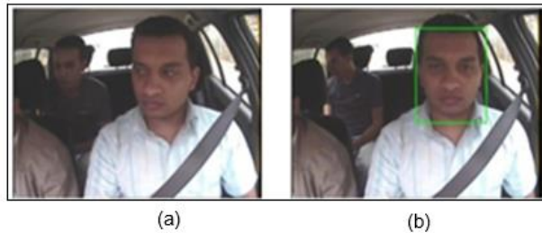
Fig 7. Verification of the frontal position of the face. (a) Face is not accepted for tracking (not-frontal), (b) Face accepted for tracking (frontal).
