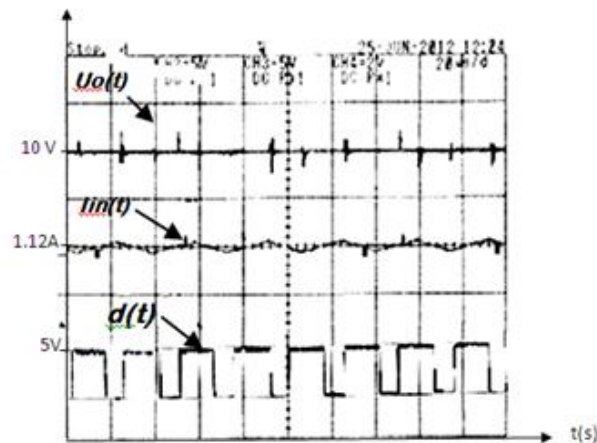
Fig. 18. Superbuck converter operation in PCM mode the output voltage, the input current, the control signal d .
