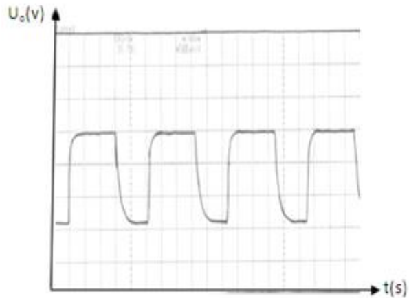
Fig. 16. The output voltage of the Superbuck controlled converter VMC driven by a photovoltaic source.
