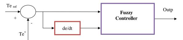
Fig. 9. Fuzzy logic control of torque hysteresis controller.
