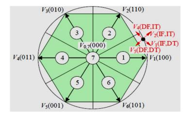
Fig. 2. Different vectors of stator voltages provided by a two levels inverter, (100): (1: inverter switch is ON, 0: for OFF) I(D) F: increase (decrease) of flux magnitude, I(D) T: increase (decrease) of torque.
