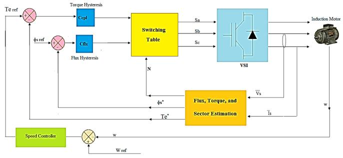
Fig. 1. Direct torque control scheme.
