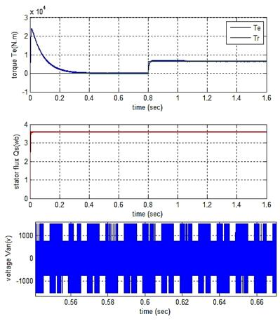
Fig. 12. Performances of classical DTC for IM.
