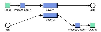
Fig. 6. Structure of neural controller.
