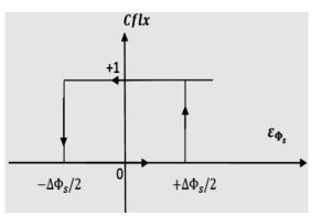
Fig. 4. Flux hysteresis comparator.
