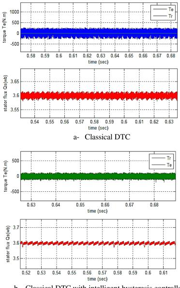
b- Classical DTC with intelligent hysteresis controllers. Fig. 14. Zoom in the flux and torque.
