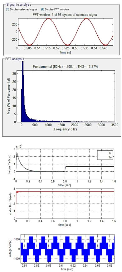
Fig. 13. Performances of classical DTC with intelligent hysteresis controllers.
