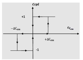
Fig. 3. Torque hysteresis comparator.
