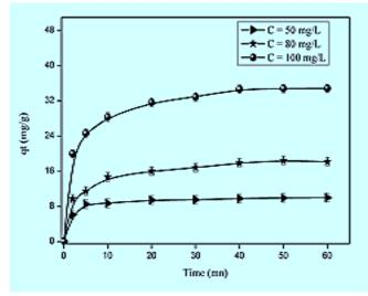
Fig. 3. Effect of contact time on the adsorption onto ASAC.
