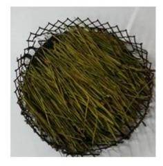
Fig. 1. A view of *Pinus halepensis* needles in the sample holder of 10cm diameter and 5cm height.
