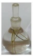
Fig. 3. The pycnometer used in measurement.
