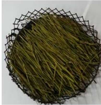
Fig. 1. A view of Pinus halepensis needles in the sample holder of 10cm diameter and 5cm height.
