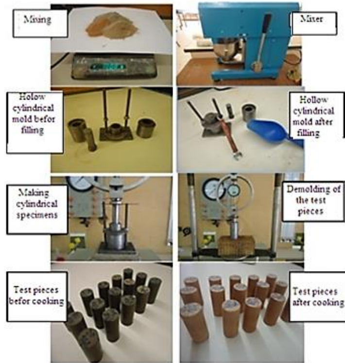
Fig.3. Preparation in laboratory test pieces of the brick.
